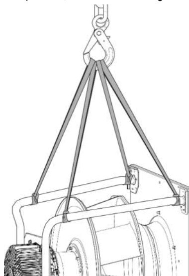
Fig. 1: Hoisting diagram for transportation of RadiPac
