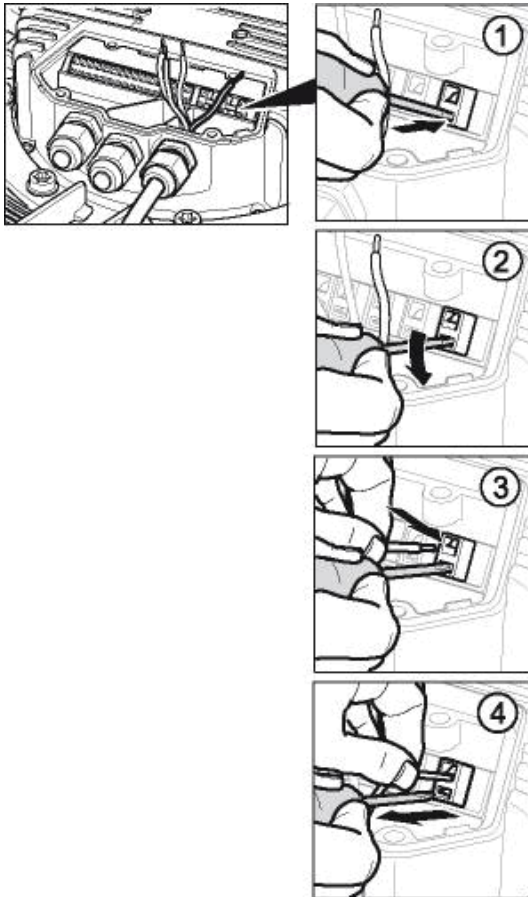
Fig. 2: Connecting the wires to terminals
